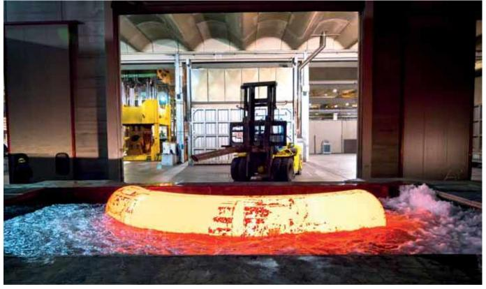
Above: some processing phases of large tee fittings Below: hot elbows in the large cooling tank during the heat treatment process
