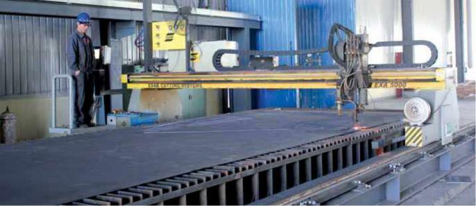
Checking of plates and precision cutting with CNC Oxy-Plasma machine. Thicknesss up to 110 mm
