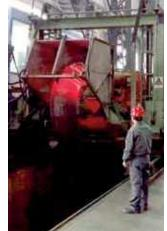
The larger mandrel bending: 900 tons pushing capacity, elbows up to 44" and bends (3D, 5D, 7D) up to 44"
