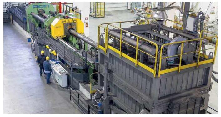
Gas mandrel and bending machine MTC 450
