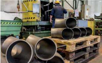
Above: the cold forming machine in the Podenzano plant for the production of tees up to 16" Below: the cold bending machine in the Calendasco plant for the production of elbows up to 16"
